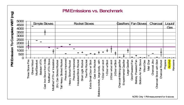
4.) Chimney Stoves Emissions Exemption: Wood burning stoves with chimneys are exempt from the above standards if the stove does not allow more than an average of 50 parts per million of Carbon Monoxide to pollute the air anywhere within 30 cm of the stove. Exempt stoves with Chimney shall use less than 1500 grams (30,000 kJ) of fuel to boil and simmer for 45 minutes 5L of water according to the Shell/UCB revised water boiling test.
